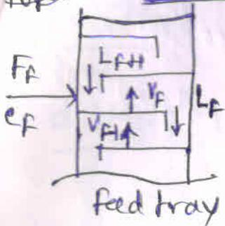
$$\frac{d(M_F)}{dt} = F_F + L_{F+1} + V_{F-1} - L_F - V_F$$
