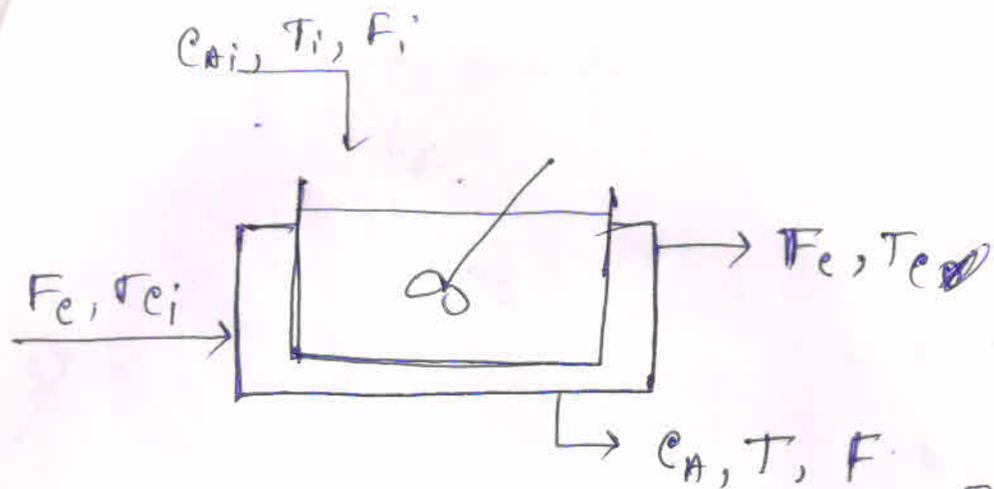
$$\frac{dc_A}{dt} = \frac{F_i}{V} (c_{Ai} - c_A) - k_0 e^{-E/RT} c_A$$
